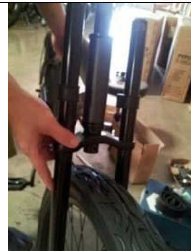
4) Insert fork into center tube
