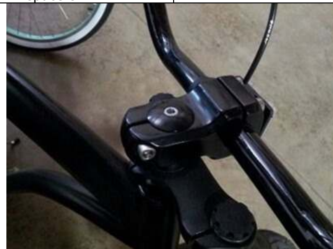
15) Insert stem and handle bar than insert the final cap with bolt tighten.
