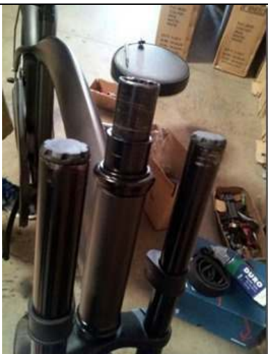
13) insert 2 spacers than last O ring
