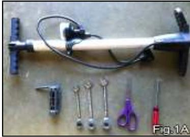
2. Assembling your brand new beach cruiser will take approximately 15-20 minutes. Following these step by step instructions will help make the assembly process faster and easier. To begin, your beach cruiser will arrive in a box. The tools that are needed to assemble the bicycle are a tire pump, an allen wrench with variable sizes, Phillips head screw driver, scissors, 10-15mm C wrench. Please see fig. 1A.
